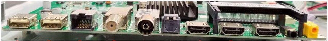
USB 2.0-1 USB 2.0-2 RF (S2) RF (T/T2) AV/optical HDMI1 HDMI2 HDMI3 AV IN Earphone
